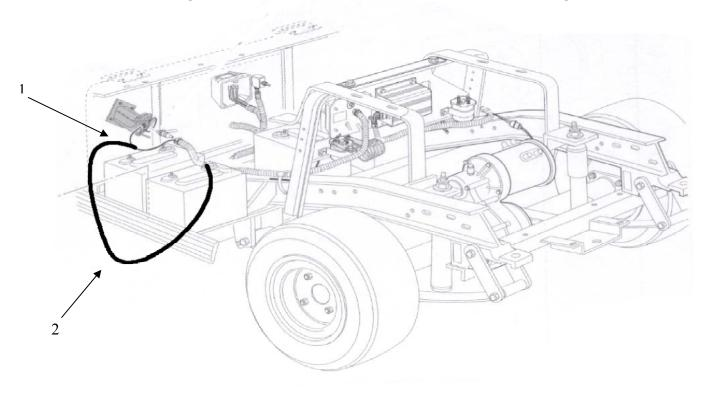
Your Club Car has an on-board computer for the single purpose of turning on or off your Club Car charger. When the batteries are fully charged this computer tells the Club Car charger to remain off. Or when the batteries are in need of charging this same computer tells the Club Car charger to turn on.
