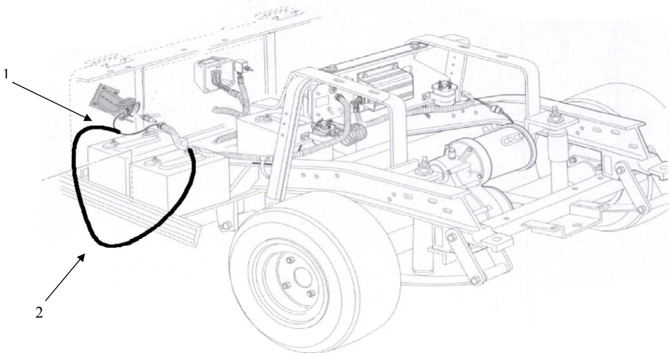
Your Club Car has an on-board computer for the single purpose of turning on or off your Club Car charger. When the batteries are fully charged this computer tells the Club Car charger to remain off. Or when the batteries are in need of charging this same computer tells the Club Car charger to turn on.
